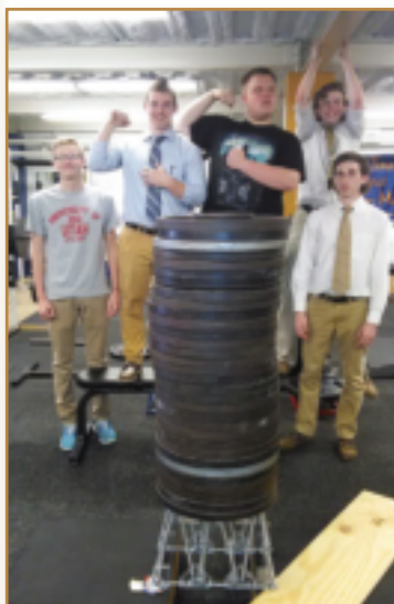
The winning team in Brother Baginski's Engineering I class designed and constructed this bridge of Aluminum and acrylic that held 1,540 pounds.
